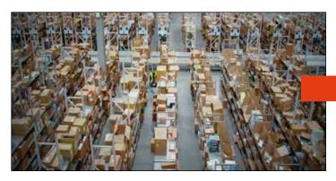
On racking, a standard pick is a minimum of a 5m round trip and picking from the furthest point would be a 20m round trip.
