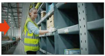
Storeganizer is installed right next to the conveyor belt, the picking distance to the first row of pick faces is only 1m
